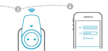
Plug NEO Switch into a power outlet, then press ON/OFF button for 5 seconds and release it The Wi-Fi indicator light will flash quickly. NEO Switch is now ready for synchronization.
